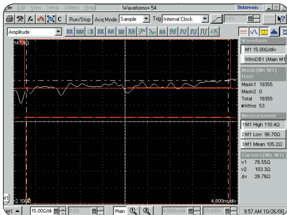
► Figure 18: USB 2.0 impedance measurement, outside specifications (mask displayed)
